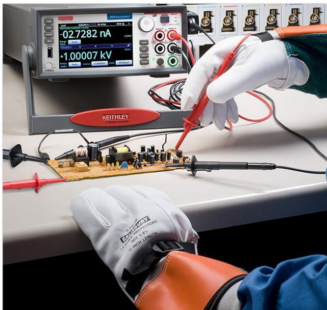
Figure 11. Using proper safety gloves when working with high voltages on energized components.
