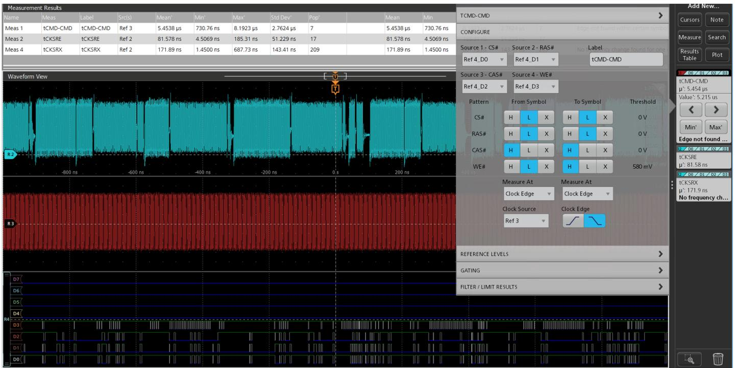
Configuring DDR3 digital measurements using TLP058 probes.
