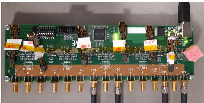
FIGURE 7. D-PHY termination board, with TriMode probes soldered in place.
