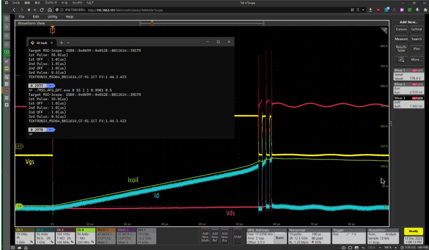
Figure 12: 3-Pulse DPT, parameter rounded.
