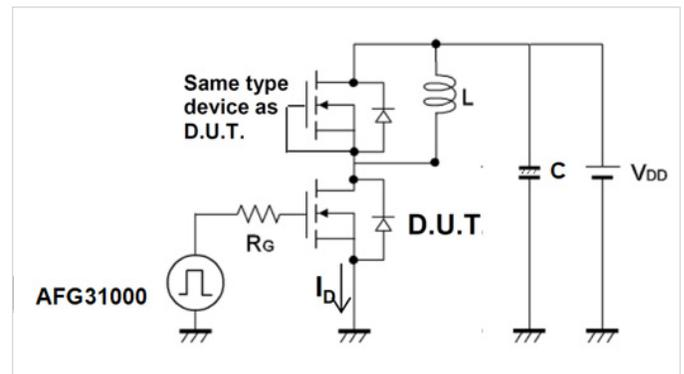
**Figure 2:** In low-side DPT testing, the high-side FET is turned off and the low-side FET is switched. This simplified setup shows basic signal flow. In an actual test setup the function generator feeds an isolated gate driver. **Figure 4** shows a more detailed circuit.
