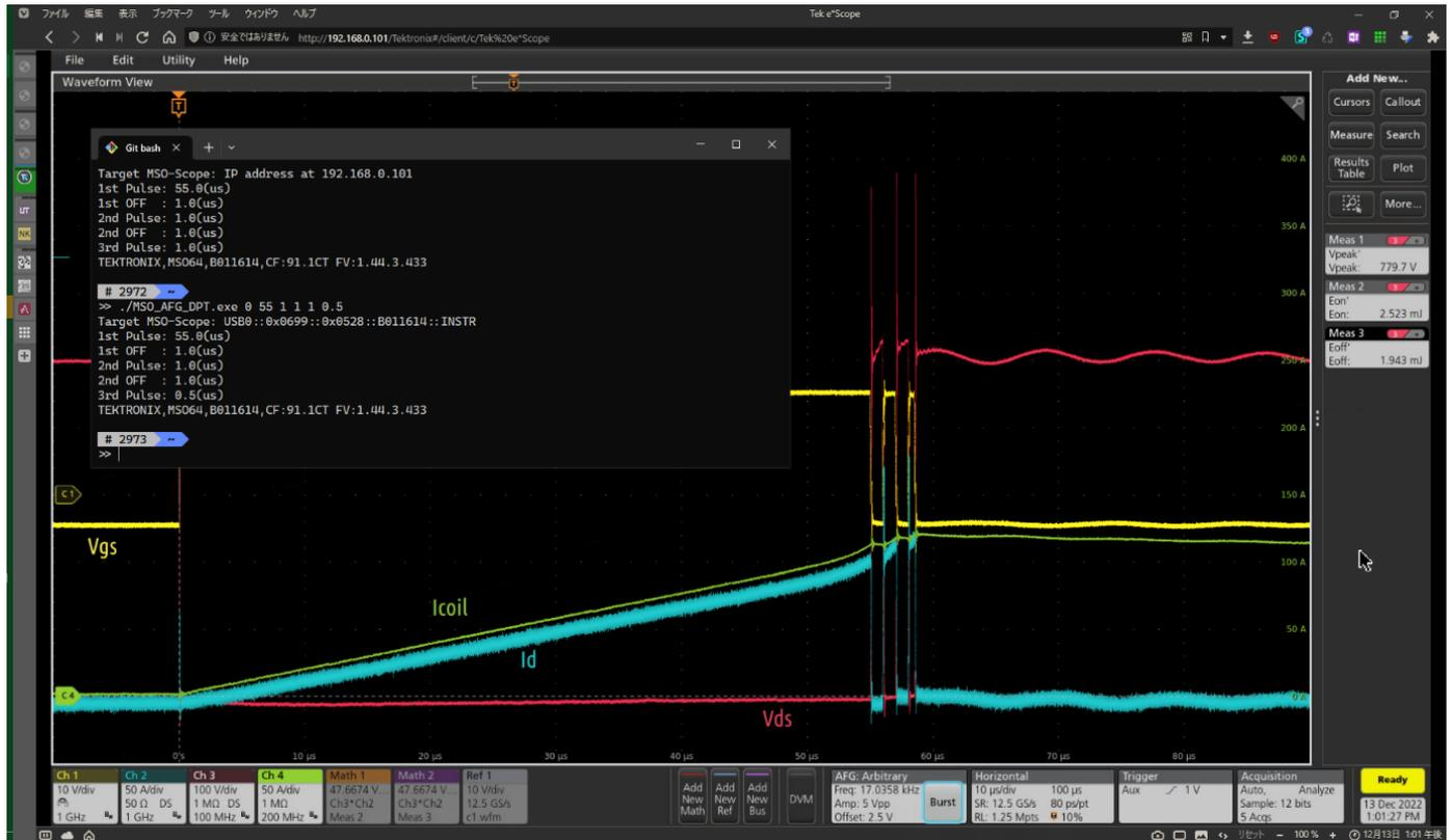
Figure 11: 3-pulse DPT with 100 ns resolution. The third pulse is 0.5 µs wide. When compared to the test in Figure 10, one can see that the third pulse is half as wide.
