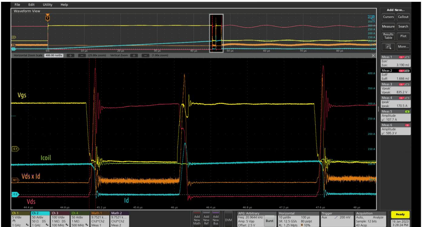
Figure 15: Zoomed in waveform shows 3-pulse DPT results.  $V_{DS\_peak}$ ,  $I_{D\_peak}$ ,  $E_{ON}$ , and  $E_{OFF}$  measurements calculated using the WBG-DPT software on the 6 Series MSO are shown in measurement badges.
