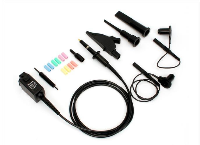
Figure 5. Tektronix TPP0850 Voltage Probe. Single-ended, ground-referenced probe with 50x attenuation (up to 100V<sub>RMS</sub>) and 800 MHz bandwidth.
