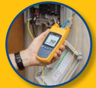
Test at the optical network terminal (ONT or hub)
