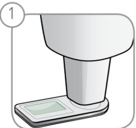
1 Position RaySafe ThinX on a flat surface. Position the collimator of the X-ray machine close to the sensor area.
