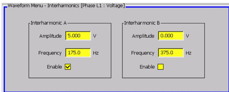
Interharmonics are a requirement to meet the multicondition testing situations in IEC 61000-4-30 and IEC 61000-4-34.
