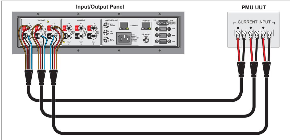
**Figure 4-3. Voltage Connections (Three Sets of Voltage Shown)**
