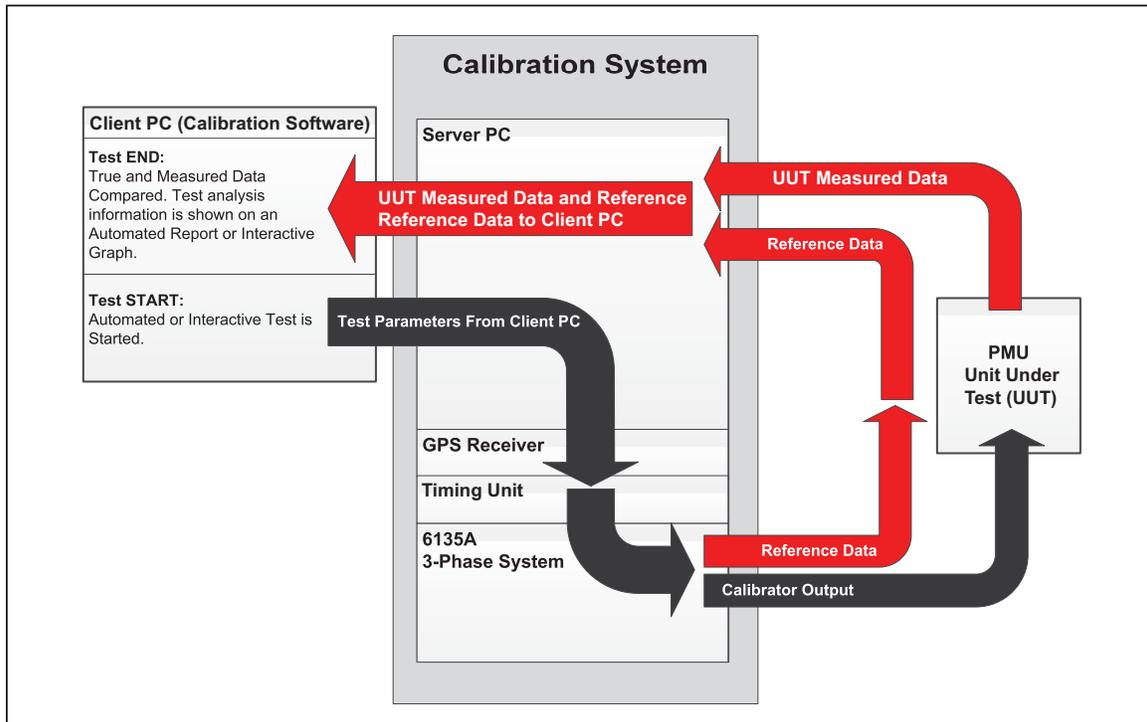
Figure 3-2. How the Calibration System Calibrates a UUT
