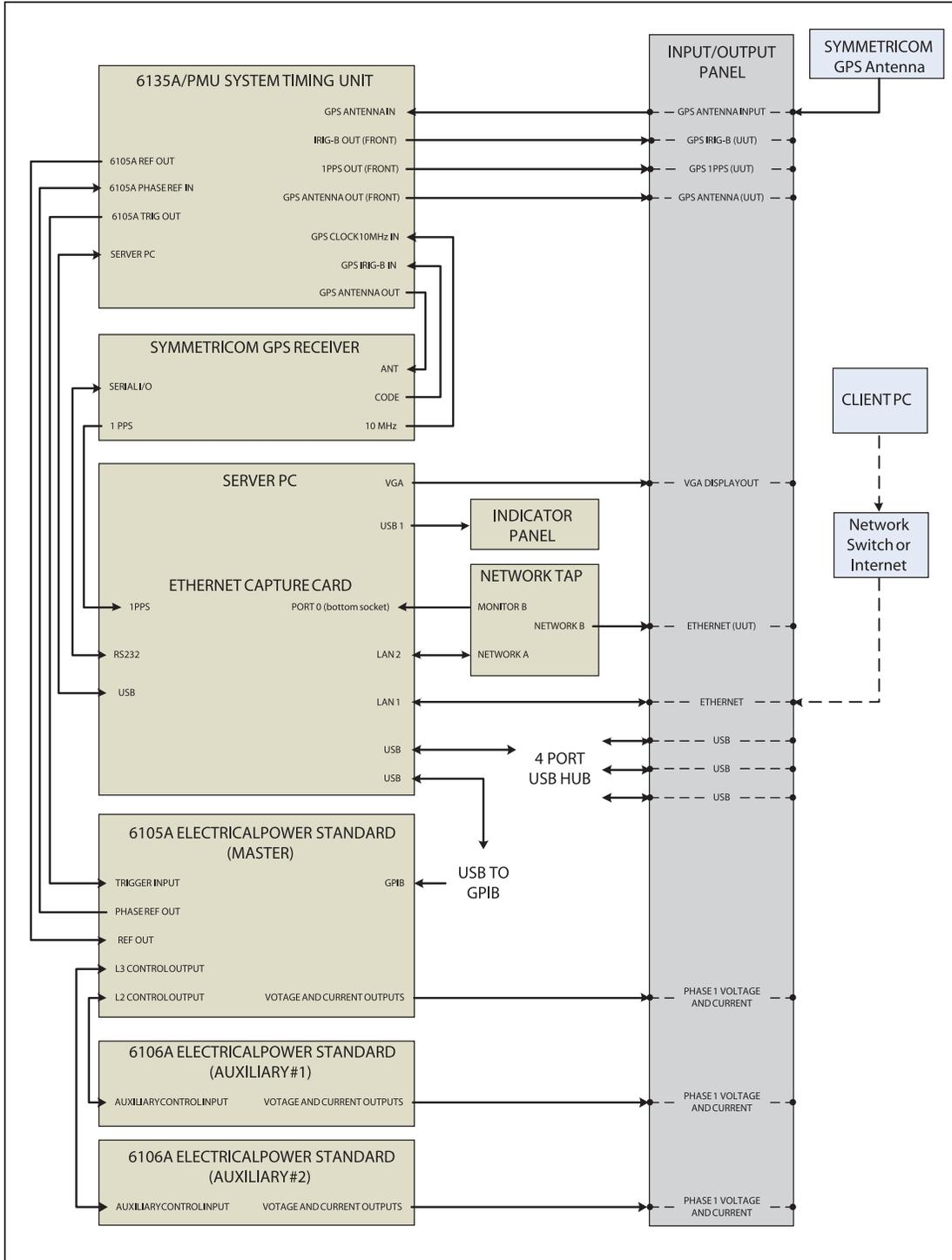
Figure 8-1. System Connections
