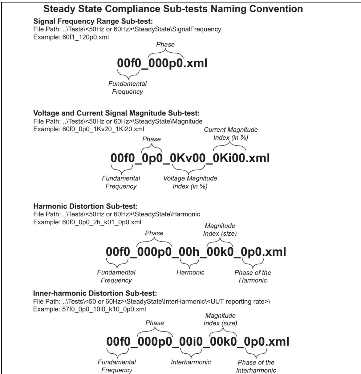
**Figure 3-18. Steady State Compliance Subtest Naming Convention**
