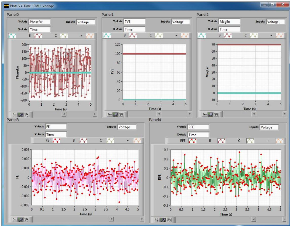
Figure 4-10. Problem - Voltage Phase B is Not Connected
