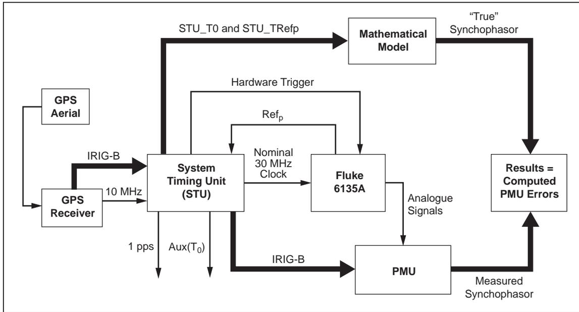
**Figure 3-5. Simplified Block Diagram of the 6135A/PMUCAL**
