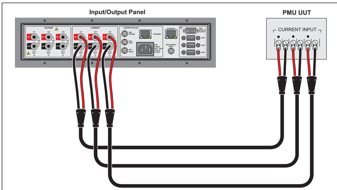
Figure 4-2. Current Connections (Three Sets of Current Shown)
