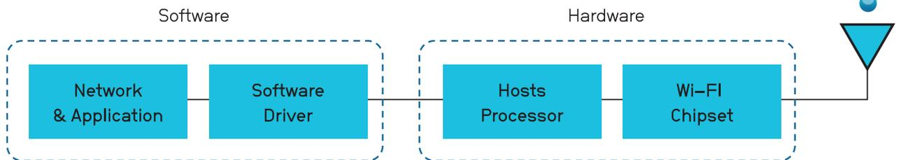
Figure 2. Simplified Block Diagram of a Typical Wi-Fi Module
