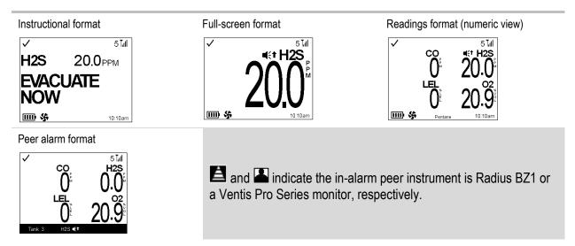
Figure 6.4 Alarm and peer-alarm display-screen samples
