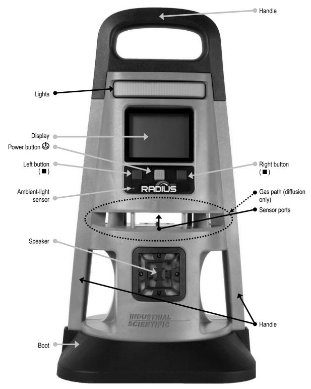
Figure 3.1.A Hardware overview Radius BZ1 (front view; diffusion)
