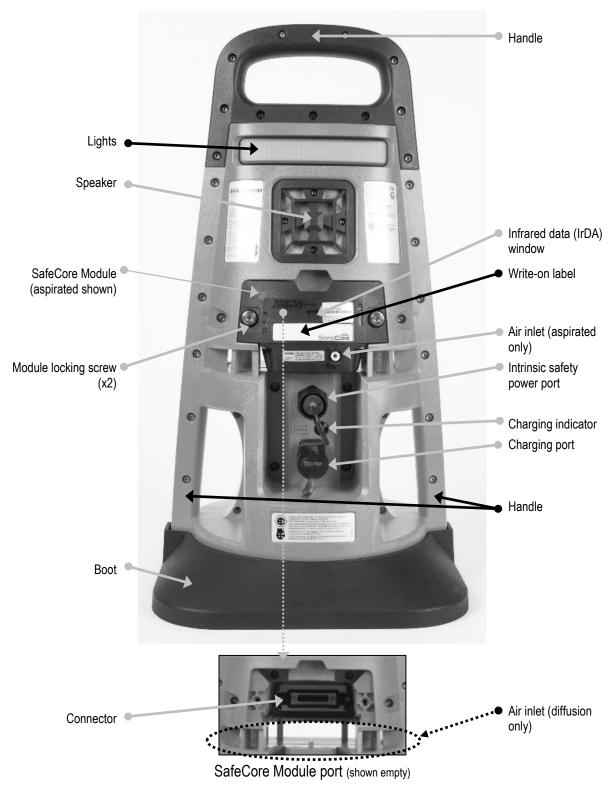
Figure 3.1.B Hardware overview Radius BZ1 (back view; aspirated)
