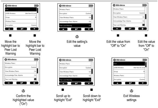
Figure 4.2 Example for editing a single-step setting
