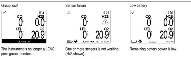
Figure 6.6 Warning display-screen samples
