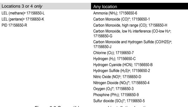
Figure 2.2 Compatible sensors and installation locations
