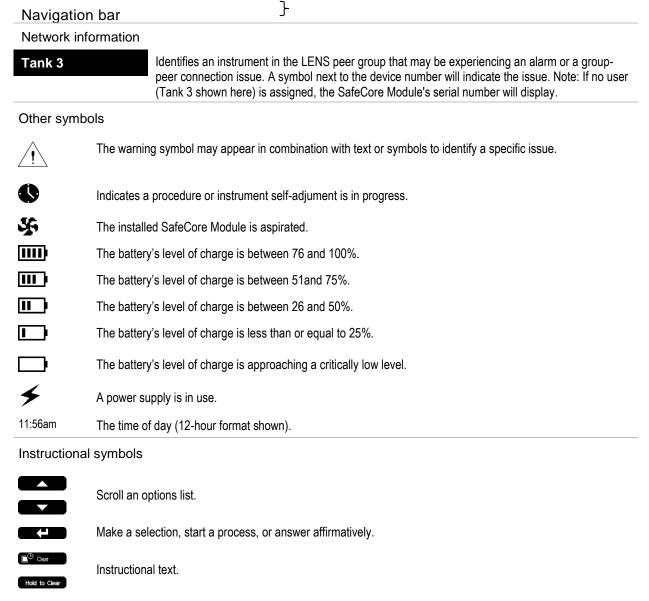
Figure 3.3 Display-screen overview during operation
