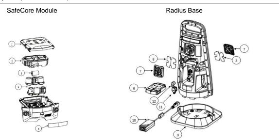
Figure 8.1 Parts diagram for SafeCore Module and Radius Base
