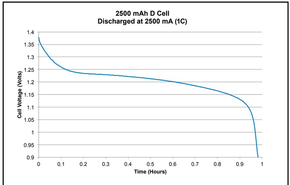
Figure 5. Discharge characteristics of 2500mAh D cell battery.
