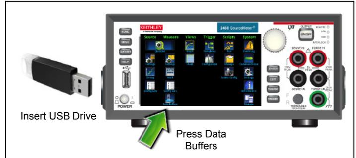
**Figure 7.** Saving data to a USB drive.
