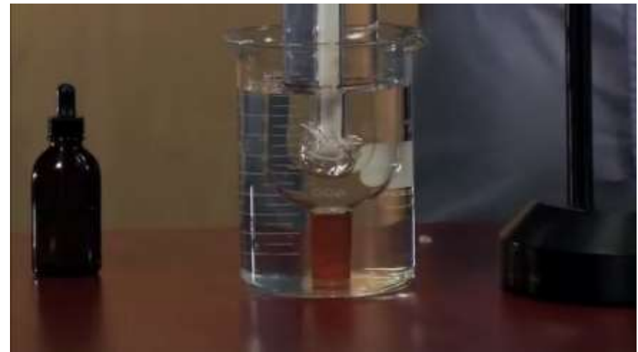
Place the cell in a Cup of water to eliminate the parallax and measure exactly the thickness of the ice mantle
