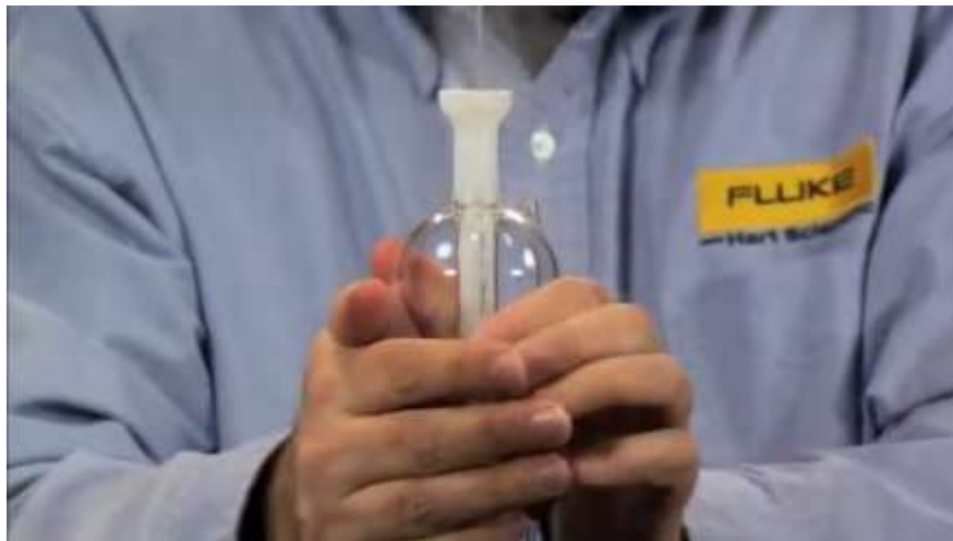
Prevent the formation of an ice bridge that may break the cell by heating this ice bridge
