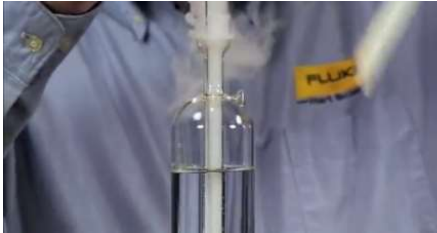
With dry ice fill the cell to form a coat of ice
