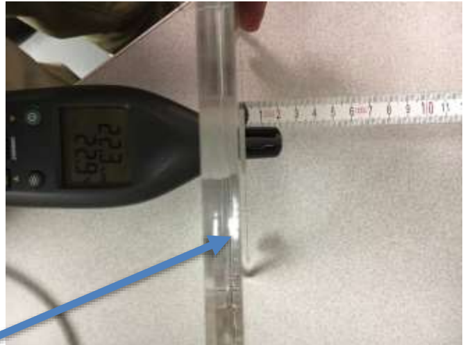
Thin door allows 2 cm of sensor immersion
