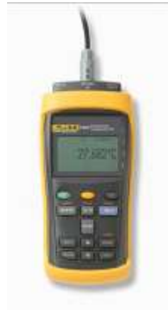
1524 with 5611T thermistor probe. System Accuracy: 0.015 °C (TAR for 2626-H cal: 8.3)
