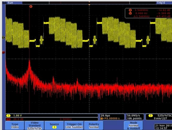
NTSC - Spectrum Analysis, peak at 3.546 MHz
