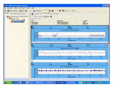
PCR measurements. The TSCA is also able to display PTS Arrival Interval graphing in real time or deferred time, and includes PTS-PCR and DTS-PCR graphs to detect possible Receiver buffer under- and overflow problems.
