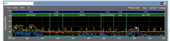
Figure 1: Visualize RF energy across the spectrum
