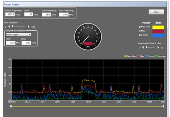
Figure 11: Verify antenna performance using the Power Meter Tool
