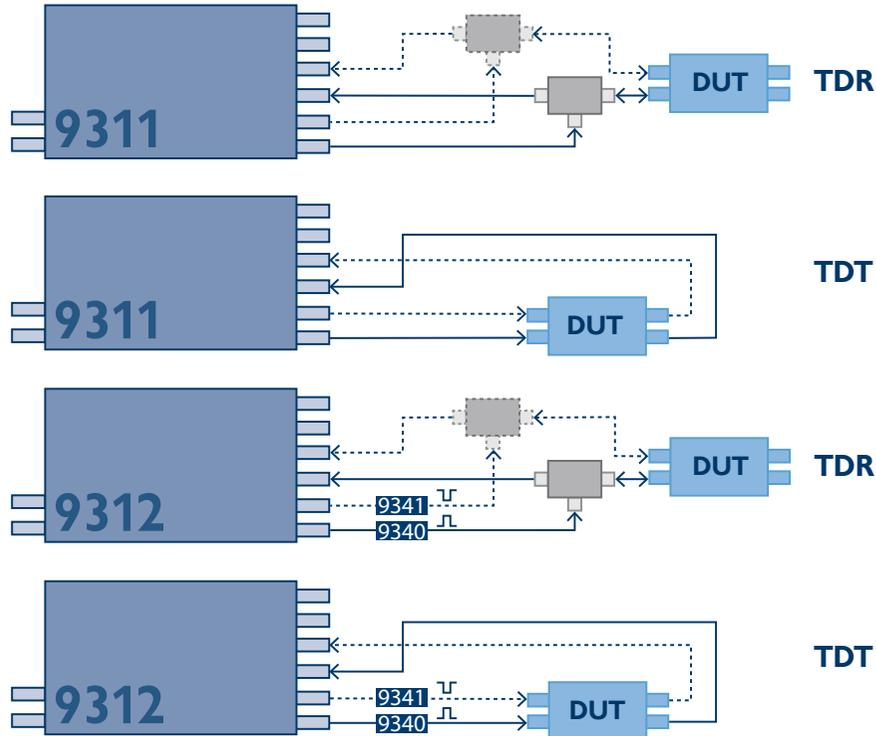
Connection diagrams: PicoScope 9311 and 9312 sampling oscilloscopes in use with devices under test (DUT) in TDR and TDT applications
