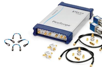
PicoScope 9312 with 9040 positive and 9041 negative pulse heads
