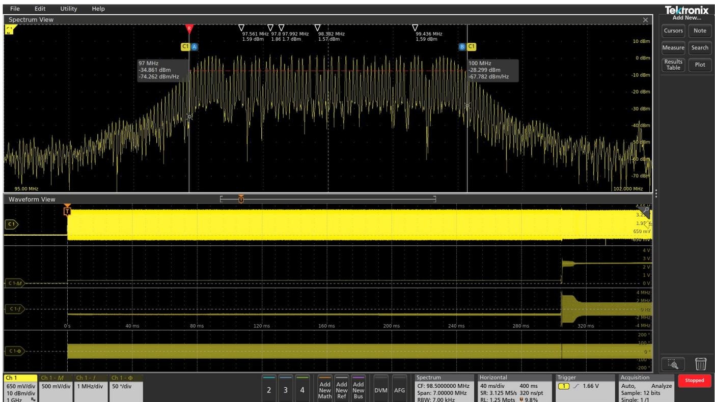
**FIGURE 10.** It's very easy to see what's going on with this spread spectrum clock by looking at the Magnitude and Frequency vs. Time waveforms. The Magnitude vs. Time trace shows the signal turning on at the trigger point at a very low level and the Frequency vs. Time trace shows the signal staying at a single frequency for the first ~300ms. At that point, we see the amplitude of the signal increase significantly and the frequency begin changing.
