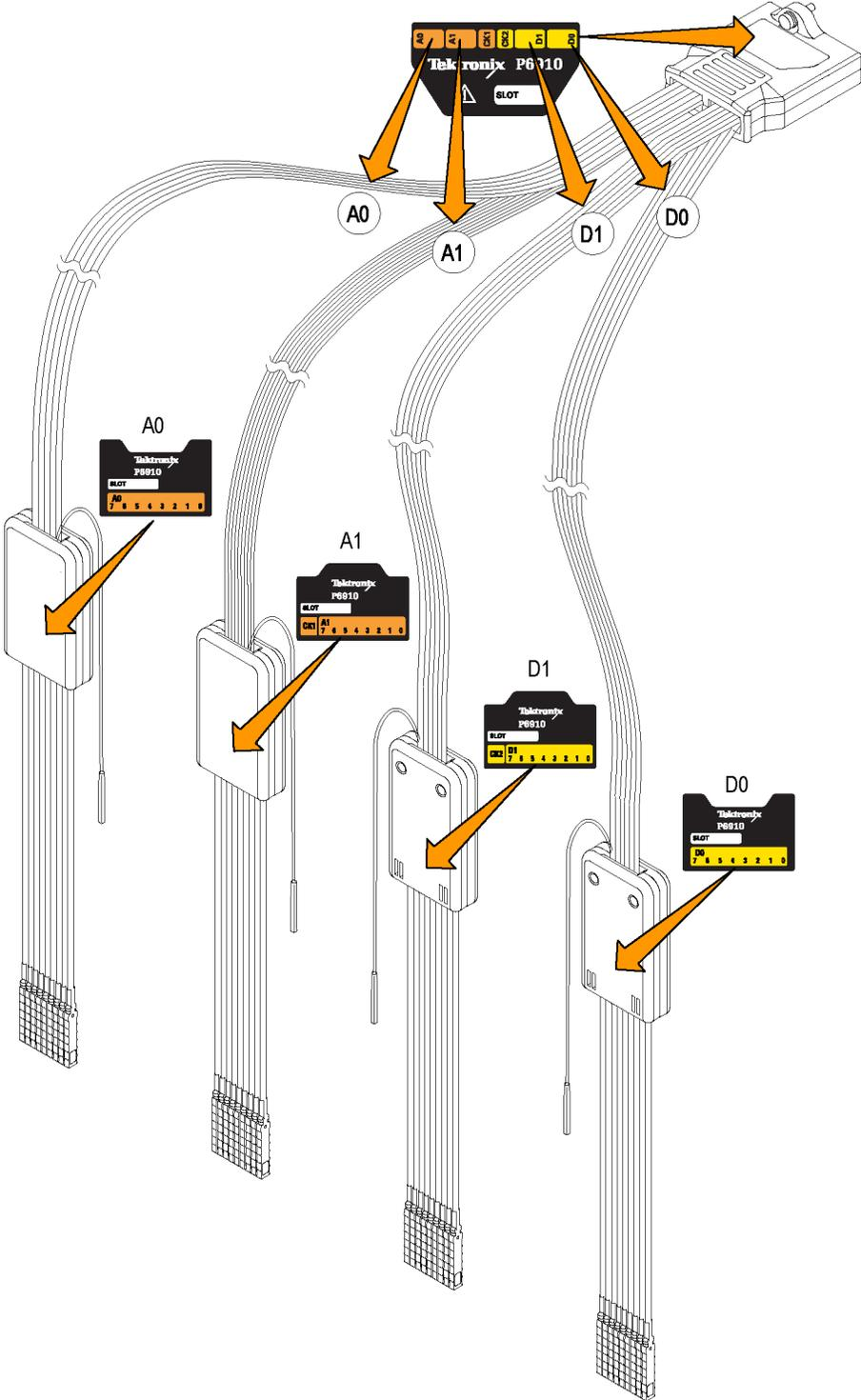
Figure 2: Attaching the probe labels
