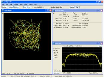
Wideband satellite and point-to-point microwave links can be directly observed with SignalVu-PC analysis software. Here, General Purpose Digital Modulation Analysis (Option SVM) is demodulating a 16QAM backhaul link running at 312.5 MS/s.
