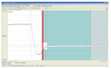
Settling time measurements (Option SVT) are easy and automated. The user can select measurement bandwidth, tolerance bands, reference frequency (auto or manual), and establish up to 3 tolerance bands vs. time for Pass/Fail testing. Settling time may be referenced to external or internal trigger, and from the last settled frequency or phase. In the illustration, frequency settling time for a hopped oscillator is measured from an external trigger point from the device under test.
