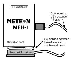
**Important:** the PS320 must be powered by the 9 V battery eliminator when using the MFA. The MFH will not be driven by the PS320 under battery power.
