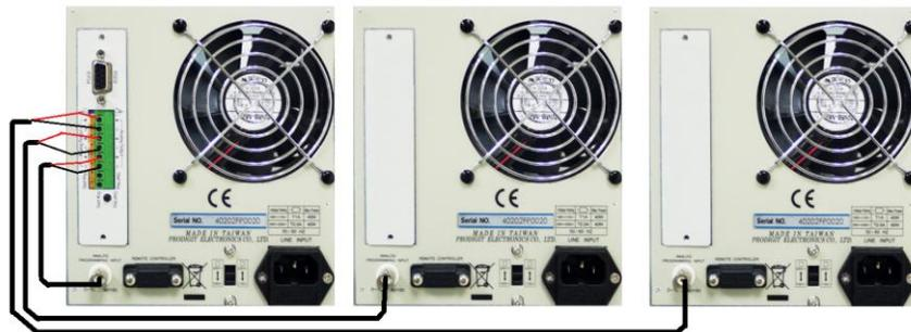
9923 is connected to three electronic loads
