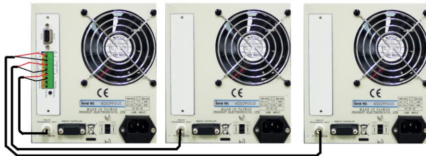
9923 is connected to three electronic loads
