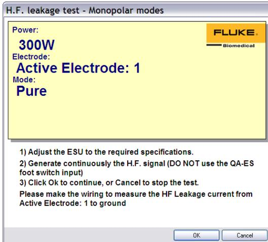
Clear instructions appear on the PC screen in large characters while performing the tests describing which electrode, what mode, and what power to set up.
