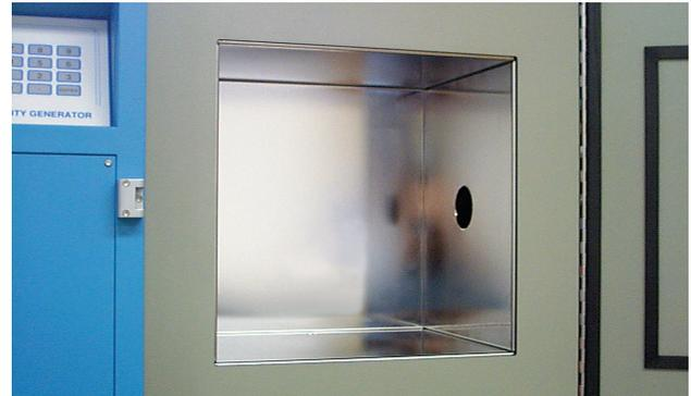
Virtually any humidity and temperature point may be generated, for any length of time, within the operational limits of the generator. The output of the device under test may then be compared with the generator's printed data for analysis.
