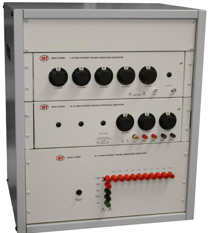
HACS-Z Capacitance Substituter: 9-decade, 10 pF through 1000 \mu\text{F} steps
