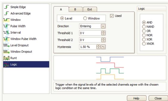
As well as the standard range of triggers found on all oscilloscopes, the PicoScope 4262 offers a comprehensive set of advanced digital triggers including pulse width, windowed and dropout triggers to help you capture the data you need.
