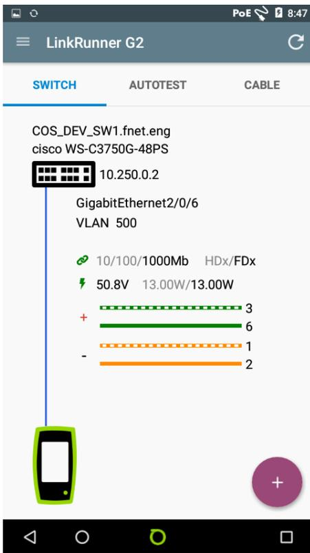
**Nearest switch and VLAN information over Copper and Fiber Links** - uses IEEE Link Layer Discovery Protocol (LLDP) plus the Cisco® and Extreme Discovery Protocols (CDP and EDP) to display the VLAN/Voice VLAN and nearest switch model, slot and port. When reported as part of the AutoTest, a Refresh option is available that allows you to receive the next xDP frame (CDP/LLDP) coming from the switch.
