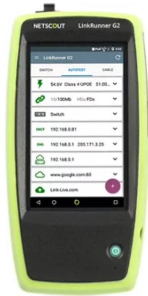
When customization of the AutoTest is needed, profiles can be defined to ensure a standardized test process is executed when variables about the link under test are needed. While these settings can be easily changed in use, profiles can be configured by a senior team member to ensure less-skilled technicians are executing an AutoTest that is specific to their network environment, which is particularly useful in organizations who manage distributed locations.
