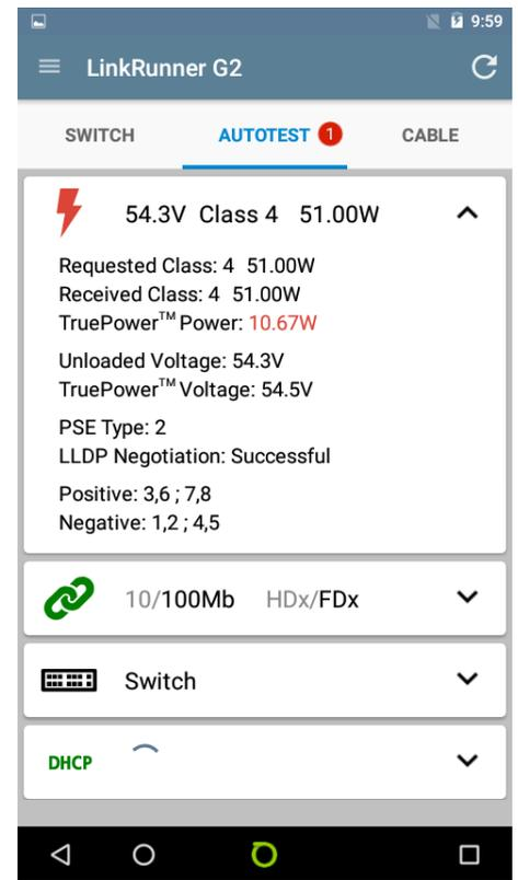
**Link Speed/Duplex** - verify link speed and duplex is configured as expected. If 1000BASE-T test is enabled and the link under test is not performing as expected, a yellow warning indication will be noted and the actual speed emphasized.
