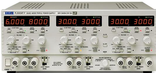
The **PL303QMT** triple has one output of 0-6V at 0-8A with 1mV and 1mA resolution. The other two outputs are each 0-30V at 0-3A with quad-mode switching providing tracking operation or true parallel to give 0-30V at 0-6A from a single output. All outputs are linear regulated.
