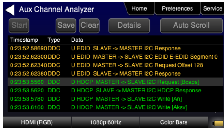
Figure 14: 780A Screen showing DDC transactions logged
