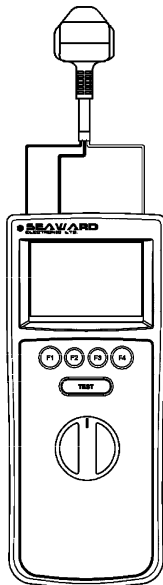
Figure 6 Mains Voltage/RCD/Earth Loop Impedance /Line Impedance Measurement
