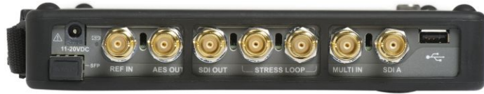
WFM2200A top panel connectors.
