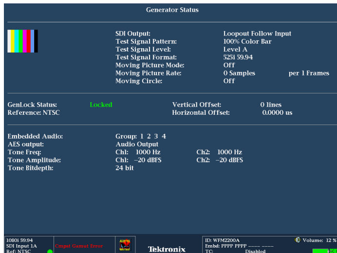
Generator Status display.
