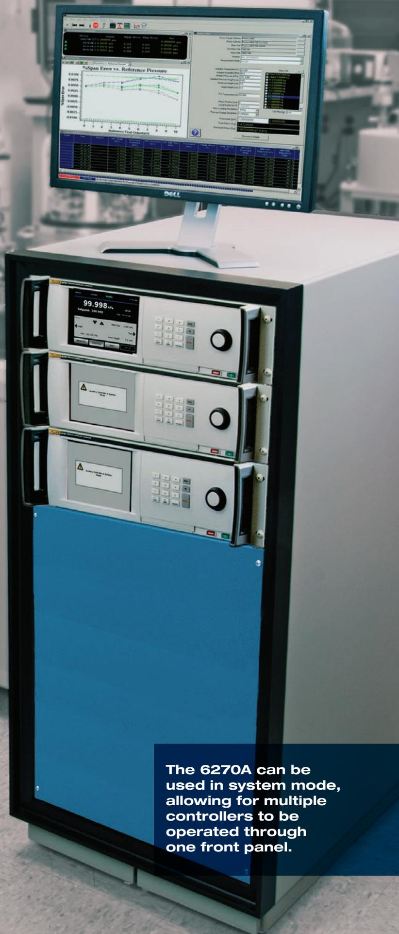
The 6270A can be used in system mode, allowing for multiple controllers to be operated through one front panel.
