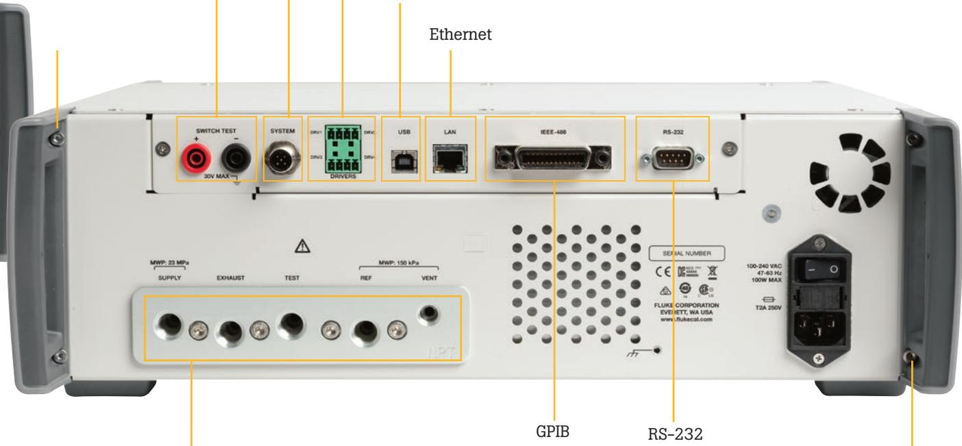
All pressure connections are located on a single, easily replaceable manifold block. Connectors in NPT, BSP, or 7/16-20 SAE enable you to choose the most popular fitting type for your region.
