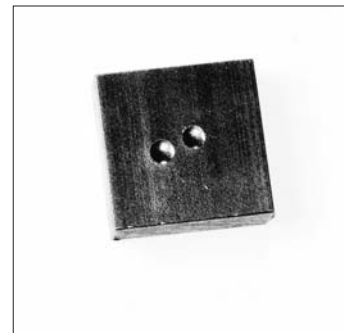
Brinell Test Piece after Brinell Indent
