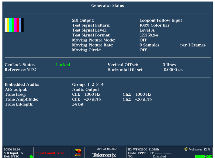
Generator Status display.
