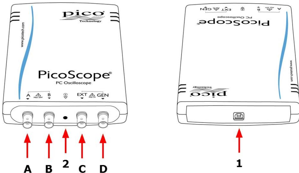
1. USB port. For best results, use the high-quality USB 2.0 or USB 3.0 cable supplied. See [Section 3](#) for guidance on USB connections.
