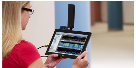
**AirMagnet Spectrum ES can scan frequencies between 698 MHz and 2690 MHz and includes support for multiple technologies.**
