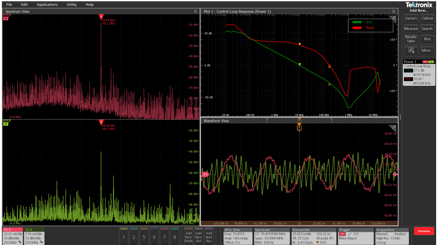
Figure 9. Bode plot (upper right) with sweep range from 10 Hz to 20 MHz. Spectrum view windows are on the left. These measurements were made on a 5 Series MSO.
