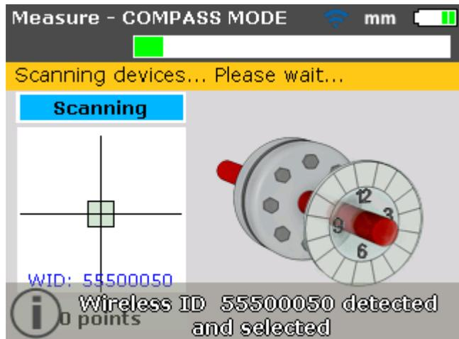
Once detected, the module is automatically connected and communication established between the sensor and the 830.
