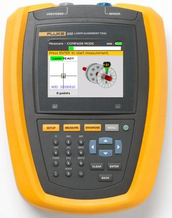
**3** Rotate shaft to first measurement position. Take measurement when sector turns green.
