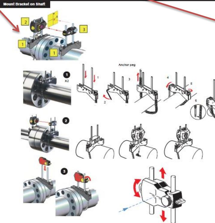
1. Mount the bracket onto the shaft.
