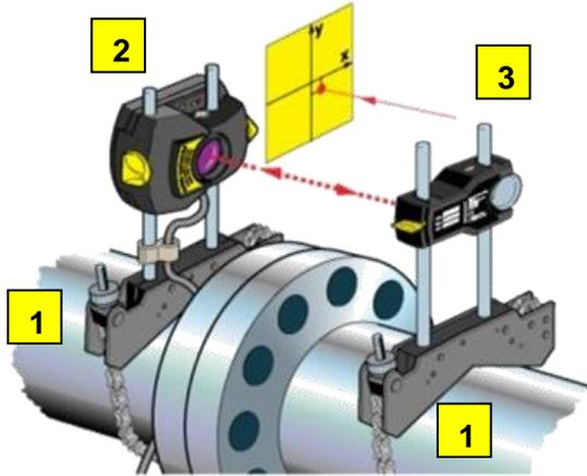
1. Mount brackets on both sides of the coupling tightly on shaft
