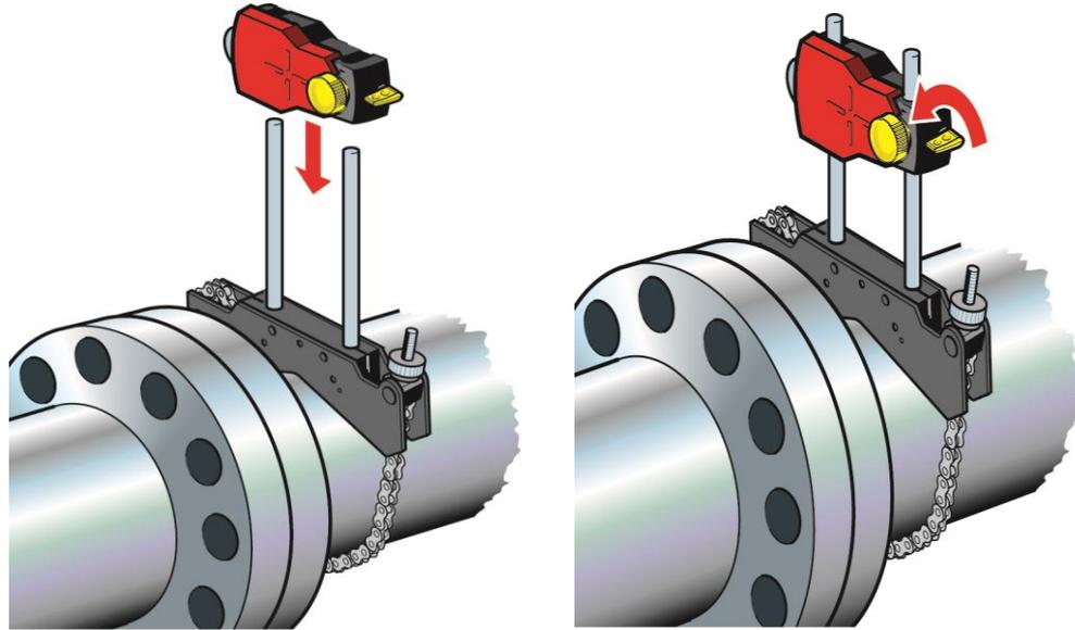
3. Mount prism on “Right machine” the same height as sensor. Center the laser dot on the prism dust cap
