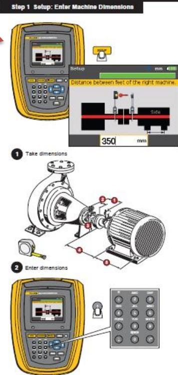
Distance between feet of the right machine: 350 mm
