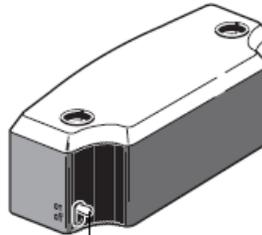
Wireless module ON/OFF switch
