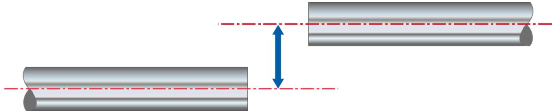
**Offset** value varies depending upon the location where the distance between two shaft rotation axes is measured
