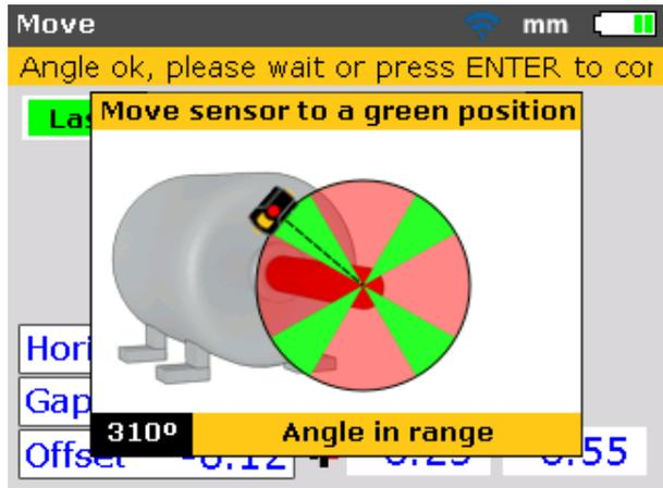
Rotate shaft to any 45° position
