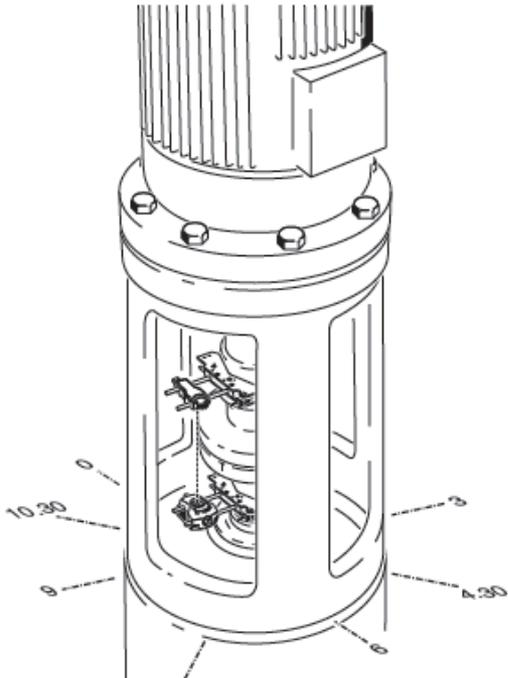
The circular housing is numbered clockwise looking down the shaft, starting at 0 followed by the clock positions 1:30, 3:00, 4:30, 6:00, 7:30, 9:00 and 10:30.
