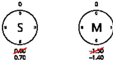
The TIR values must be divided by 2 to determine the true shaft offset values in the planes of the dial indicators:
