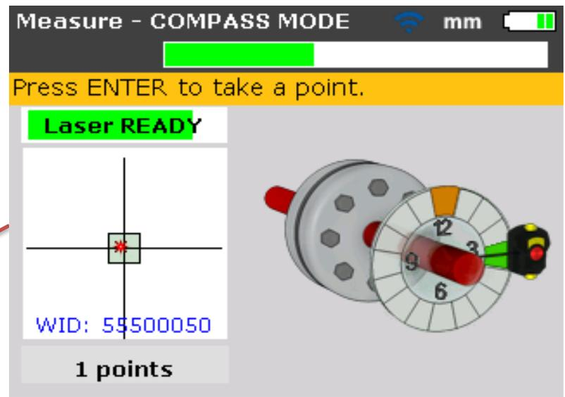
5 Take measurement #2 when sector turns green – turns orange when measurement is complete
