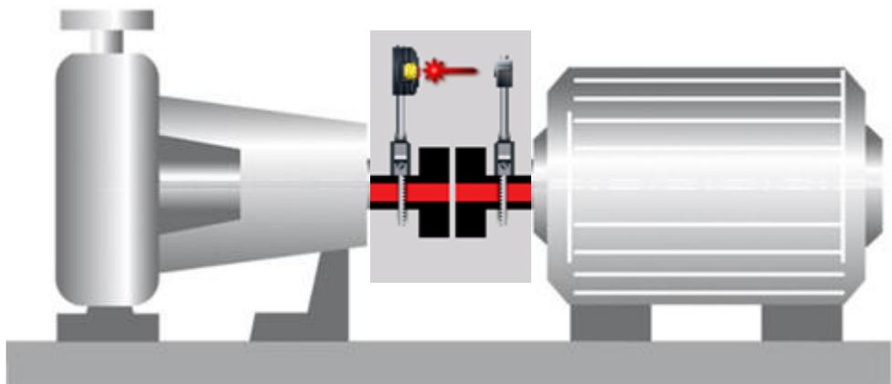
Inclinometer automatically determines angle on shaft
