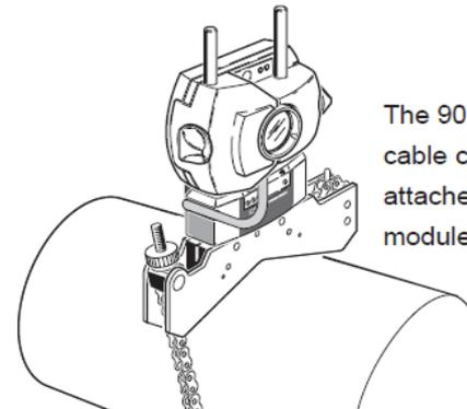
The 90-degree sensor cable connector is attached to the wireless module
