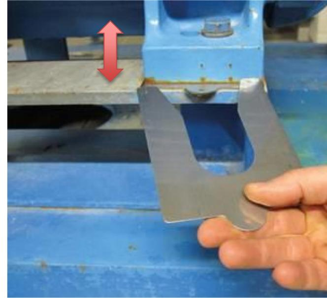
**Once alignment condition is found, a correction is recommended:**
