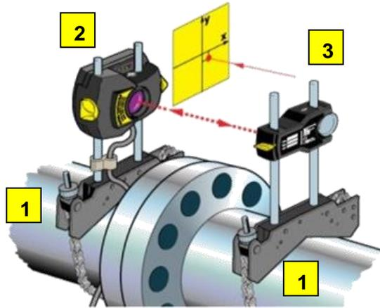
2. Mount wireless module and sensor on “Left machine” – usually Stationary
