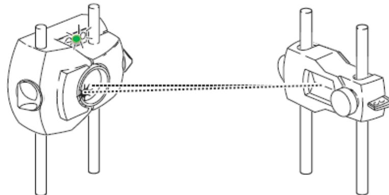
Both sensor LEDs blink quickly and alternately
