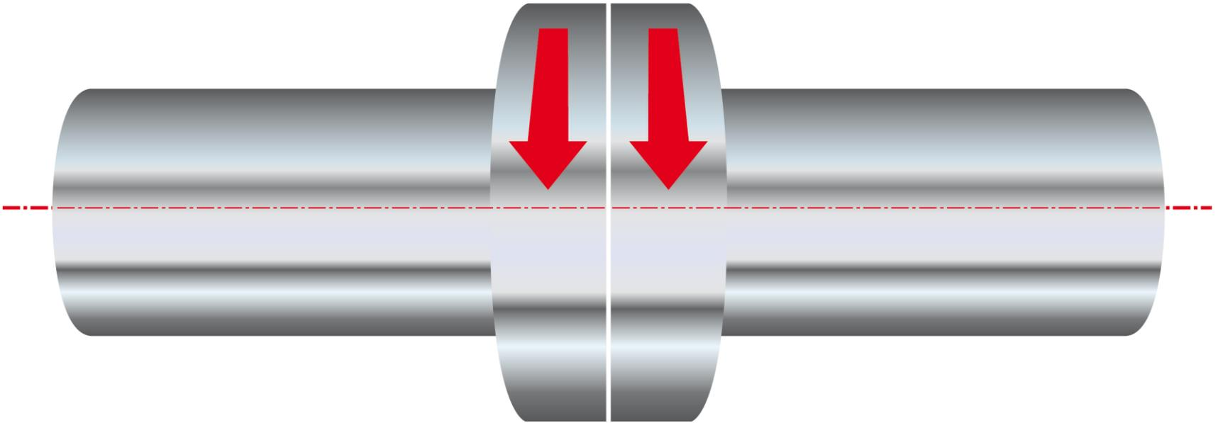
at the point of power transfer from one shaft to another, the axes of rotation of both shafts should be colinear when the machine is running under normal operating conditions
