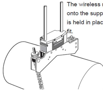
Fasten the sensor onto the support posts by tightening the yellow knobs
