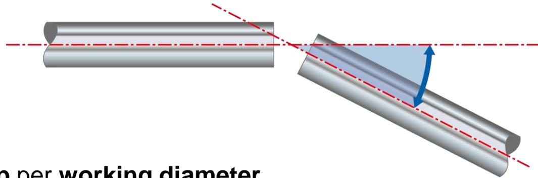
The angle is usually given as a **gap per working diameter**.
