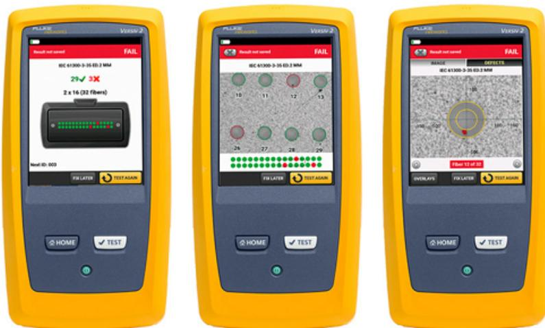
Seamlessly switch from a summary view (left) to an image (center), then use the gesture-based interface to zoom into a view of each individual fiber (right) and pan across the entire connector. Individual fibers are labeled so you know what you're looking at. Red defects are failures, green are acceptable per the selected standard.
