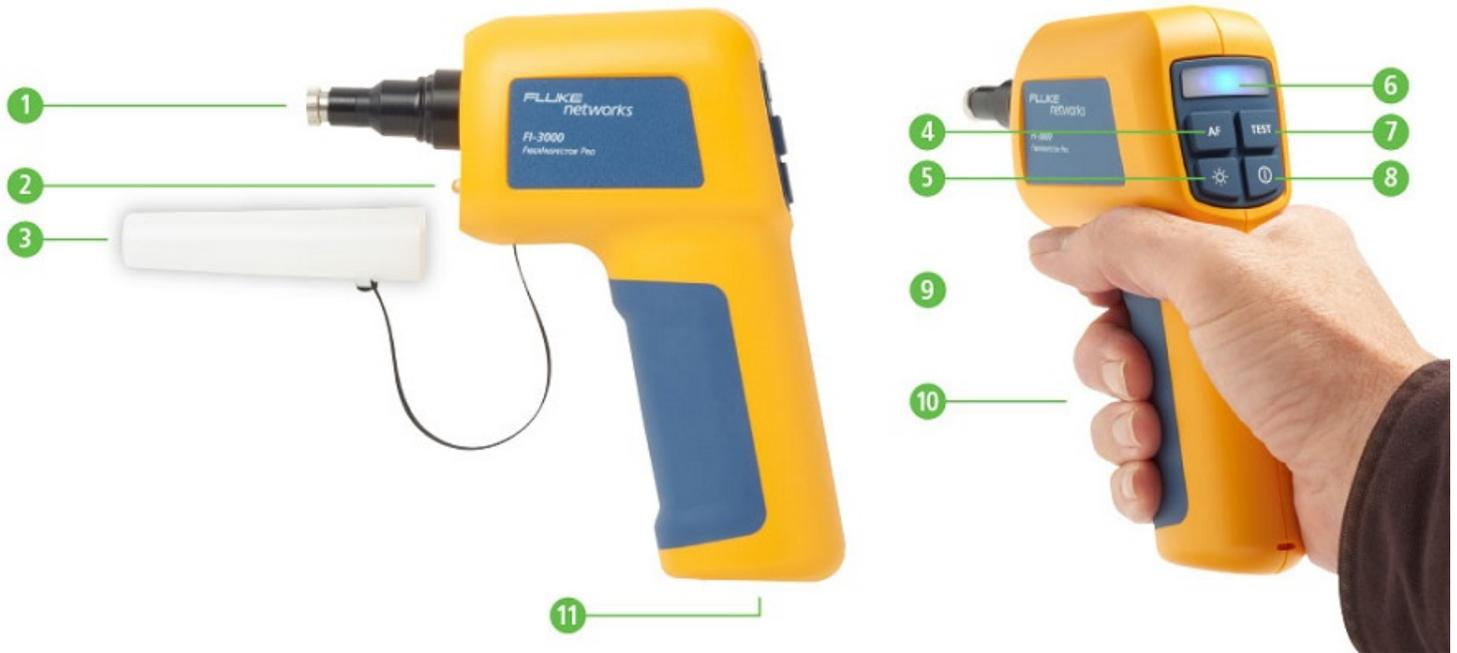
Interchangeable tips support one or two rows of 8, 12, or 16 UPC or APC connectors
