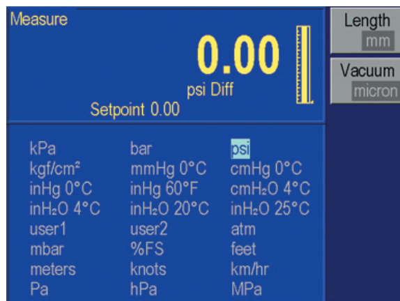
The large color display allows the pressure value to be displayed even when viewing a submenu selection such as the units selection screen shown above.
