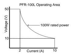
When the power supply is configured so that the total output (current x voltage output) is less than the rated power output, the power supply functions as a typical constant current, constant voltage power supply.
