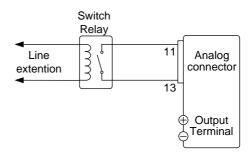
If a single switch control is to be used for multiple units, please isolate each instrument. This can be achieved by using a relay.
