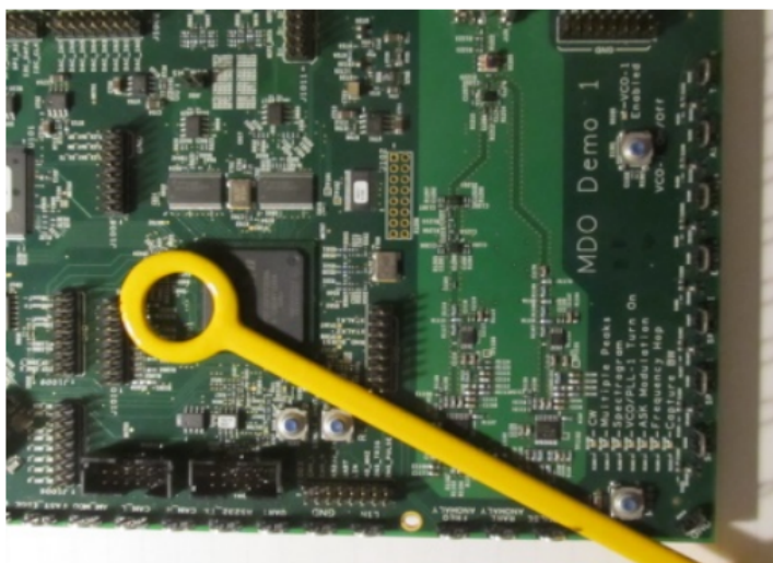
Figure 6. A Near-Field Probe Is Used to Discover the Location of Unintended RF Emissions
