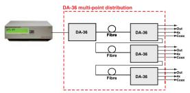
Figure 3: Multi-point distribution via cascading.
