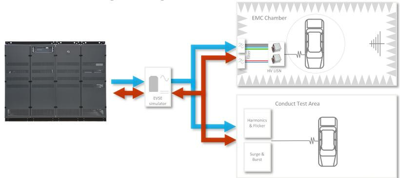
PowerWave is the ideal source to supply your **EMC chamber and conducted test area** with the power that is needed. It combines AC and DC in a compact footprint and allows charging in Mode 3 (AC) and Mode 4 (DC). With an additionally required charging station simulator (i.e. Comemso EVCA) various charging standards like Chademo, GB/T, CCS and Tesla are covered.
